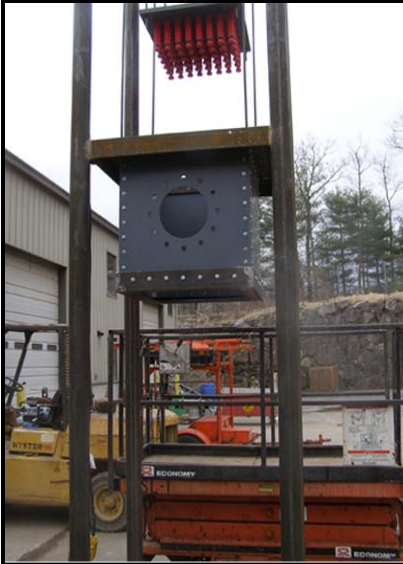
Figure 2. The Filtrex receiver with the bottom candle array visible above.
